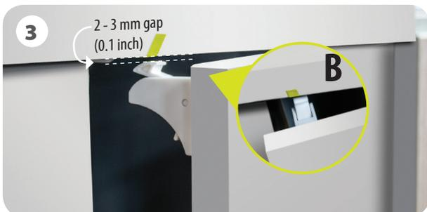
3. Install the lock body on the inside open of the cabinet door, make it 2-3mm (as shown in figure 3) distance from the bottom surface of the cabinet table, the latch hook shall be upwards, keep align center with gauge edge (as shown in figure B).
