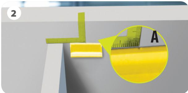
2. Paste the lock catch on the bottom of the cabinet table, keep the center groove outwards, make it alignment with the gauge angle (as shown in figure A), the location shall be parallel with the side plate of the cabinet (as shown in figure 2).
